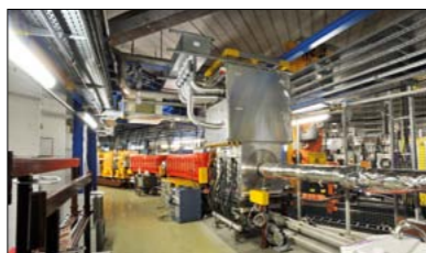
The SIS after reconstruction with the new acceleration section installed. (Image credit: Gaby Otto/GSI.)
