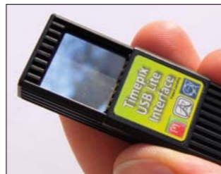
Timepix chip from CERN in a USB stick developed at IEAP, Czech Technical University, Prague. (Image credit: IEAP CTU.)
